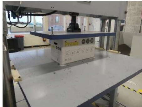
Fig. 8 – Compression test setup
