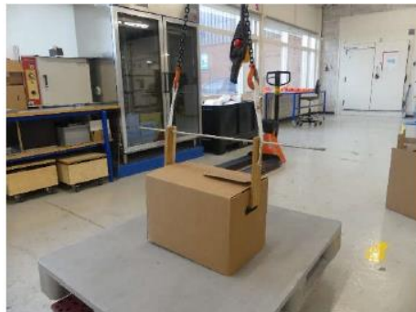
Fig. 9 – Strength of hand holes and bottom test setup
